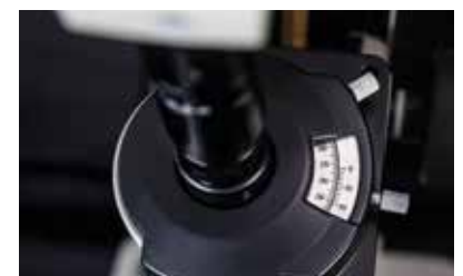
Vernier protractor incorporated at the eyepiece section of optical tube.
